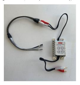
Here is what the wires from the Rockford Fosgate part look like when they are connected in parallel with the left speaker for a zone:
